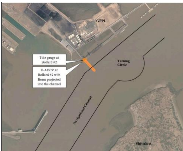
Fig. 1—Typical Installation of PMS in the Harbour
