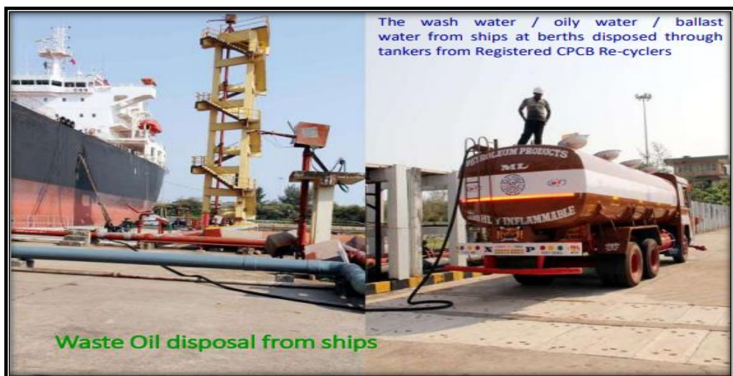
Fig 3.4 Disposal of Sludge /Bilge water from vessel to authorized KSPCB Truck [Source: - NMPA Web]
