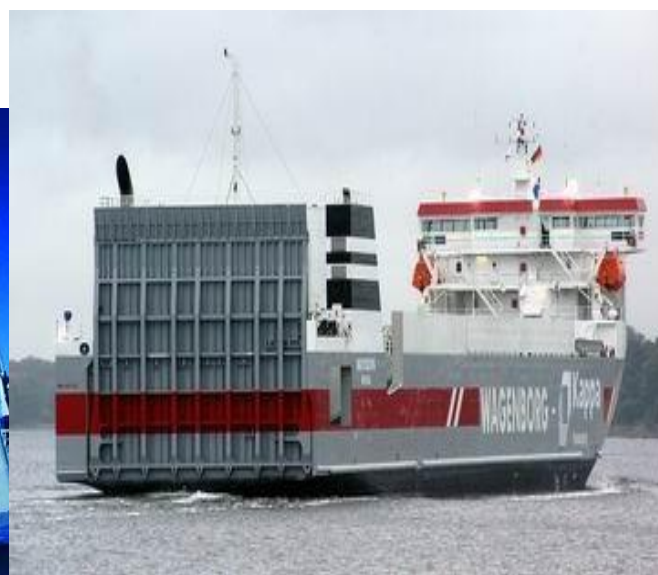
Fig 10:Ships that visit Ro/Ro terminals have stern ramps.
