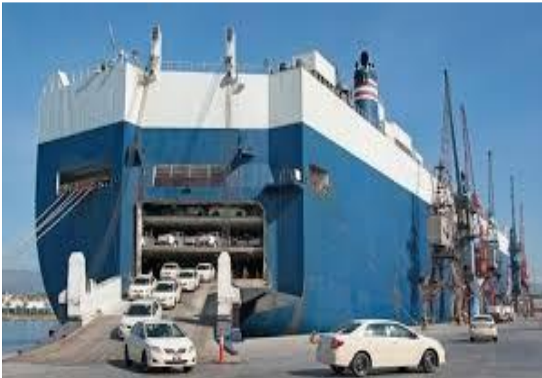
Fig 12:Bow Access Ramp
