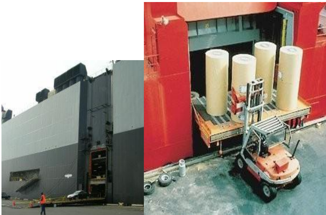
FIG 14: Side Doors of ro-ro
