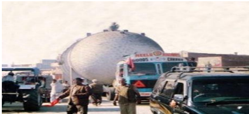
Fig 4.14 Critical Over Dimension Cargo: Length less than 40m x Width less than 6m x Height less than 5m – Weight less than 90 tons
