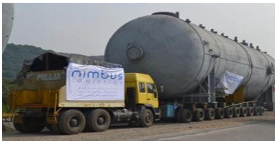
Fig 4.15 Super Over Dimension Cargo: Length less than 40m x Width less than 6m x Height less than 6m – Weight above 90 tons
