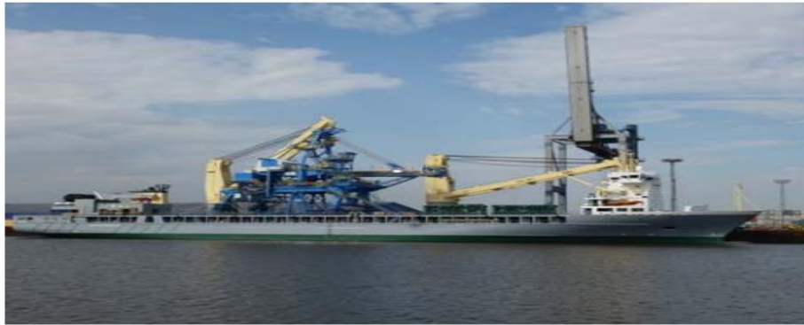
Fig 4.7 Purpose-built heavy-lift ship designed for project cargoes.
