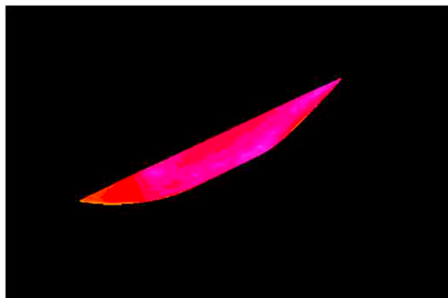
Fig. 6. Wall shear stresses of a 100 passenger vessel at a draft of 3 m and speed of 3 m/s (blue indicates regions of highest shear stress and orange that of lowest shear stress).
