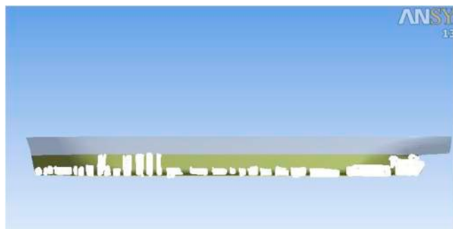
Fig. 9. Sketch of hull of predominant AF failure for tanker 1. – taken from photographs (note green indicates the underwater portion of the hull).
