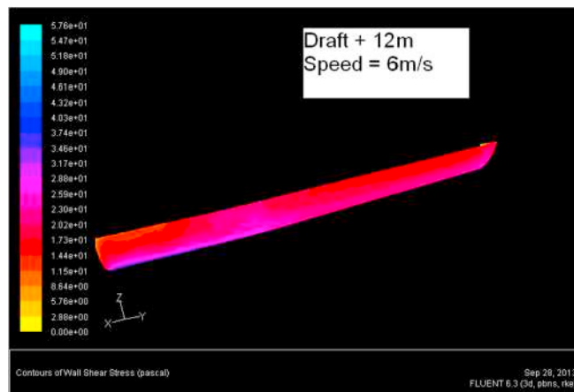
Fig. 10. Wall shear stresses of the under water portion of a tanker at a draft of 12 m and speed of 6 m/s (blue indicates regions of high shear stress and yellow the lowest shear stress) – From simulations.
