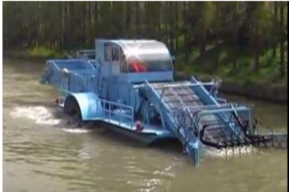
Fig1: Typical RTC (Trash Capacity 14,000 lbs)
