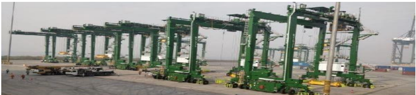
Figure 29: RTG cranes in BMCT, JN Port
