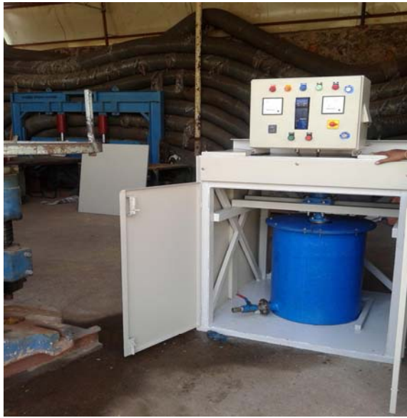
Figure 5: View of Drum Test Apparatus
