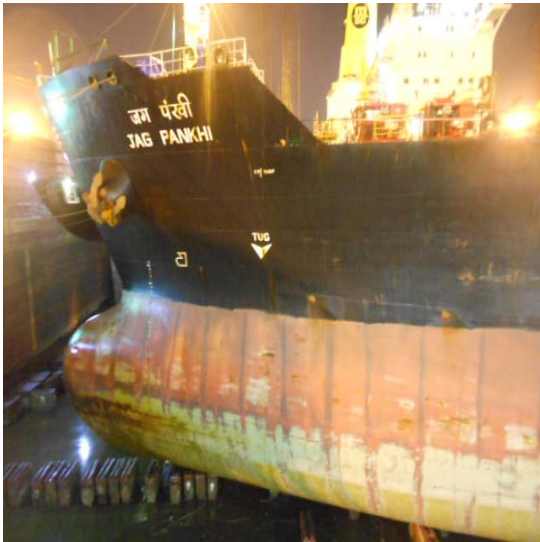
Figure 1: Photographs of a vessel taken on arrival at dry-dock indicating areas on antifouling paint deterioration
