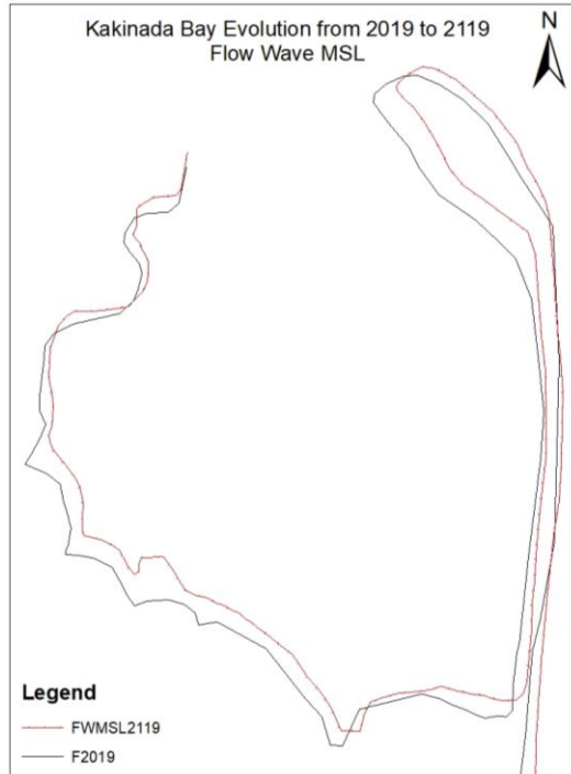
Figure 5.27. Resulting Shoreline of Kakinada Bay for year 2119 with tides and waves with MSL Rise as forcing.
