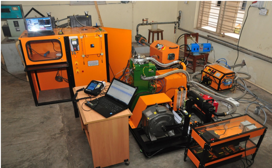
Experiment Test Rig of high-pressure multiple split injection engine test rig with exhaust gas recirculation facility.
