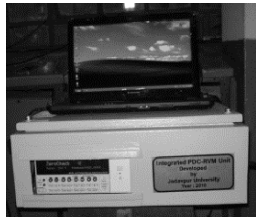
FIGURE 3. Laboratory setup for PDC measurement.
