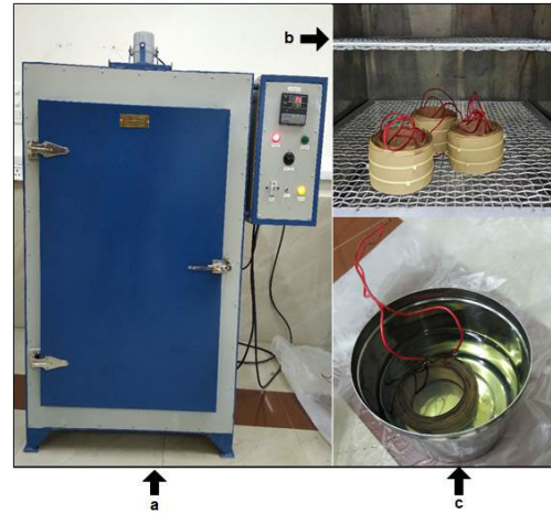
FIGURE 2. (a) Temperature Controlled Oven, (b) Drying process of samples in the oven, (c) Impregnation process of samples with transformer oil.
