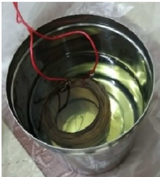
Fig. 3 Constructed test sample immersed in mineral oil
