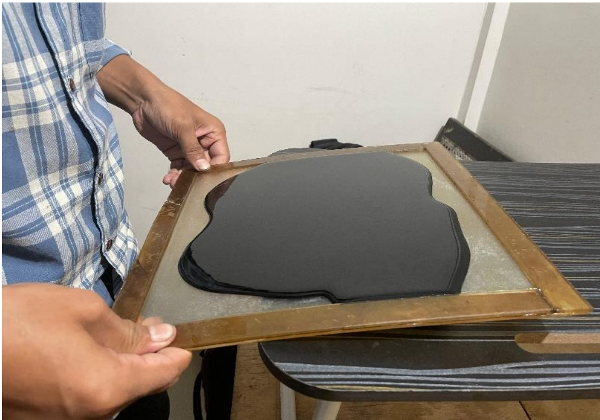
Figure 3.1 Preparation of Biochar Reinforced Epoxy Composites
