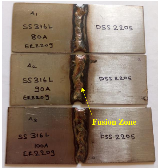
Figure 3.6: Sample after welding by using an electrode (a) ER2209
