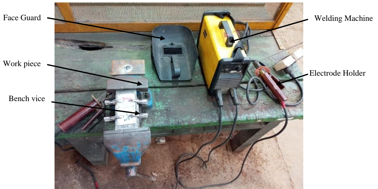
Figure 3.1: Pictorial view of SMAW welding setup
