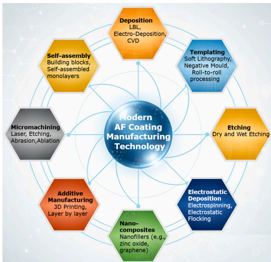
Fig. 7. Eight antifouling coating manufacturing novel techniques.
