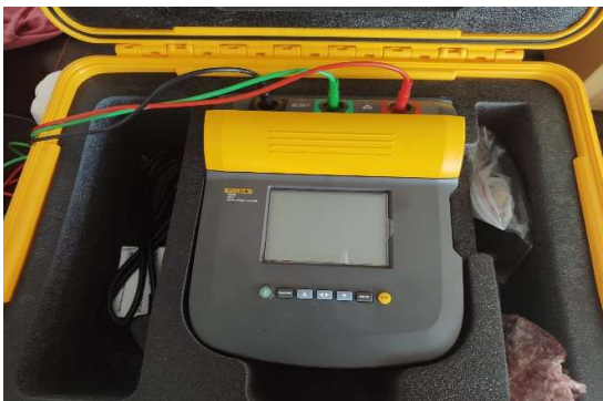
Figure- 4: Insulator Tester.
