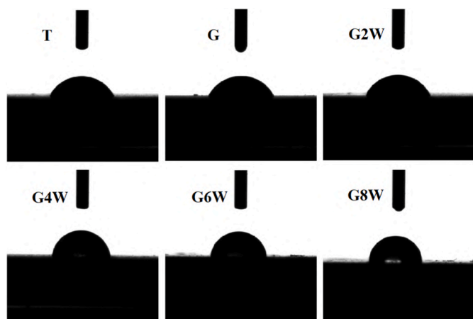
Fig. 6. Water droplet images indicating wettability of the PEO coatings.
