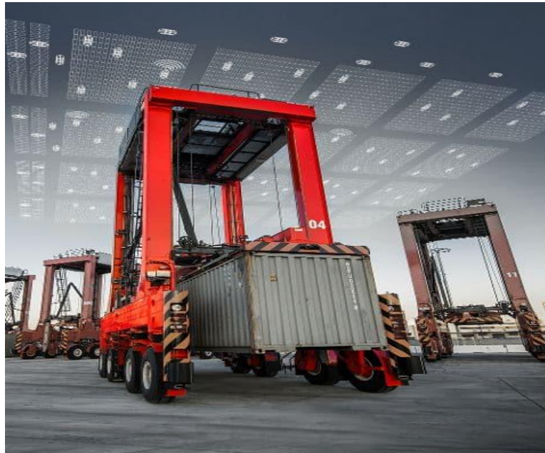
Fig3.4 Automated Straddle Carriers
