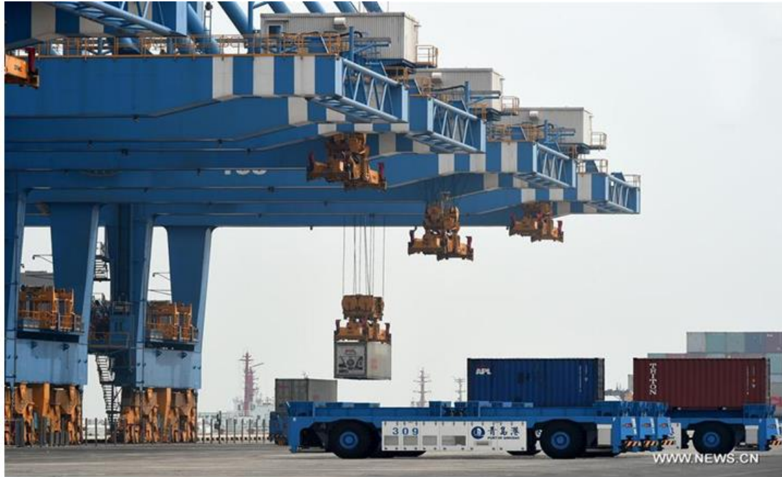
Fig 3.2 Automated Ship to Shore Crane
