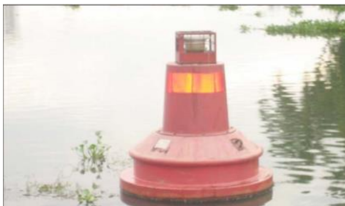
Fig 3.15 Solar Powered FRP Buoy installed in NW-3
