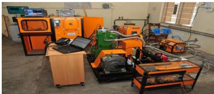
Fig.-3: Computerized Multifuel High-pressure Engine Test Rig
