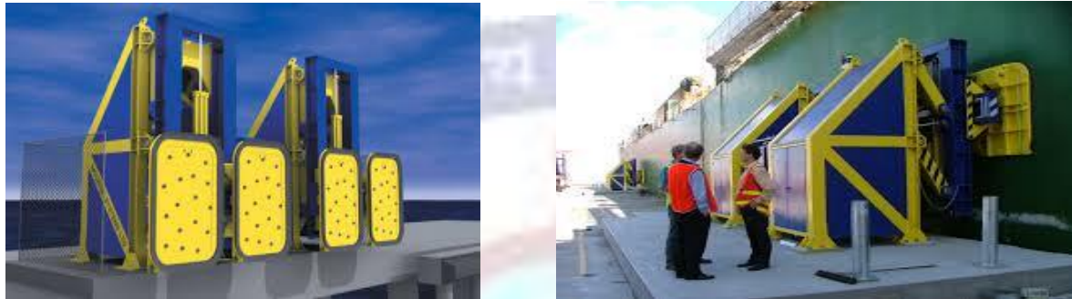
Figure 4.8 - Vacuum based mooring
