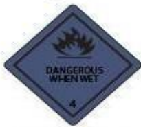
4.3-Dangerous when wet
