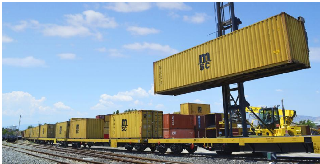
Fig. 4.7 Container Placing on Rail Wagons
